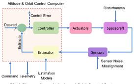
Block Diagram for an Attitude and Orbit Control System
