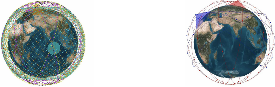
Figure 16: Planned big-LEO satellite constellations from SpaceX (left-hand side figure for 4425 LEO satellites) and Telesat (right-hand side figure for 117 LEO satellites). SpaceX proposes to have 5 different set of orbital planes at different inclination angles, whereas Telesat plans to deploy polar (red) and inclined (blue) orbits at inclination angles 99.5^\circ and 37.4^\circ , respectively. Modified from [48].
