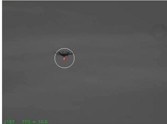
Figure 5.4: Image from the machine vision tracking camera. The red cross shows the detected position of the beacon LEDs. The white circle shows the tip-tilt mirror actuation range, centred on the predetermined hotspot.
