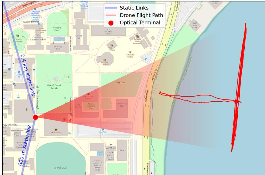
Figure 5.6: Map of flight area around the University of Western Australia campus in Perth, Western Australia. Red dot is the deployable optical terminal on the roof of the physics building, blue lines are static link paths, red line is the drone flight path during the 2022/04/21 flight. Map generated with OpenStreetMap data under the Open Database License ([openstreetmap.org/copyright](https://openstreetmap.org/copyright)).
