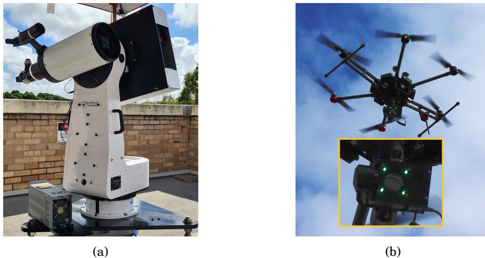
Figure 6.1: (a) Optical terminal. The upper-right box contains the free-space optics and machine vision system. The lower-left box is a tip-tilt mirror high voltage stage. The upper-left telescope is from an unrelated system. (b) Drone carrying the optical payload. *Inset*: close-up of the optical payload, consisting of LED array, pilot camera and corner-cube retroreflector.
