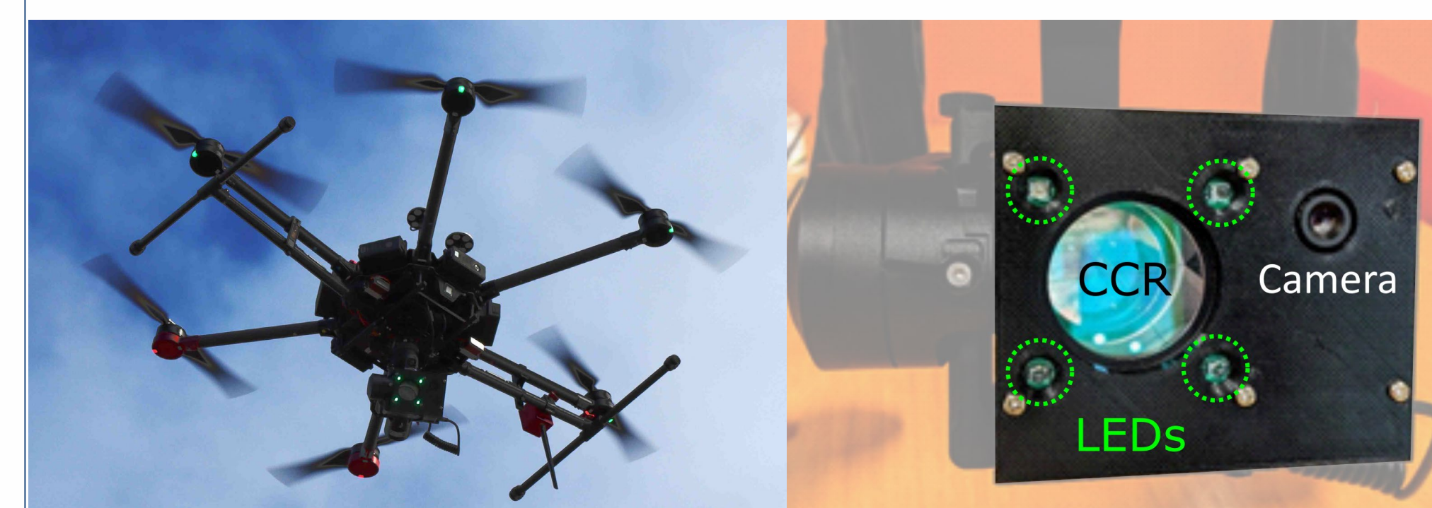
Corner cube retroreflector on drone target
