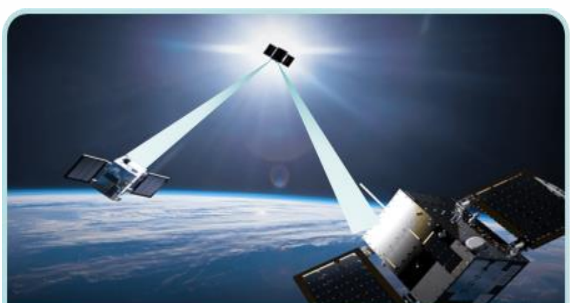
Inter-Satellite Links within a LEO satellite Cluster
