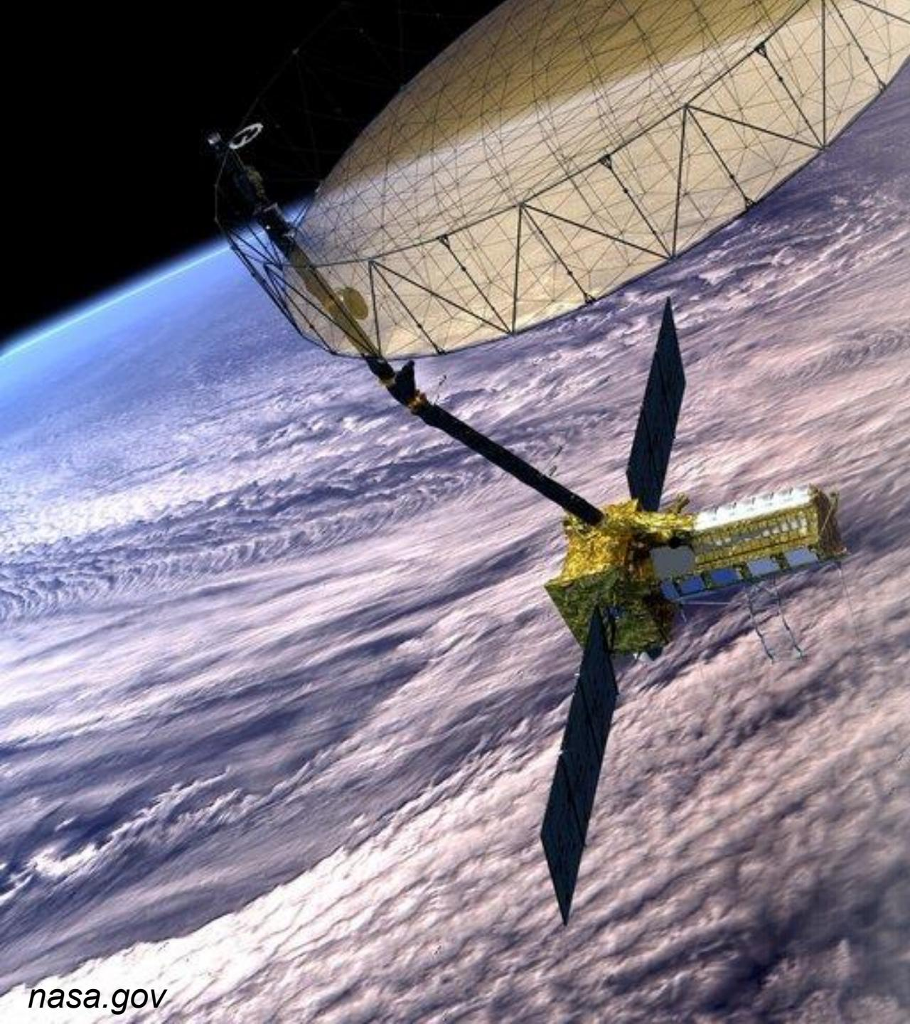
**2) Radar / Synthetic Aperture Radar (SAR)** (*Satellite sends out radio waves and measures the echo, so we can see floods and ground changes through cloud, rain and at night*)
