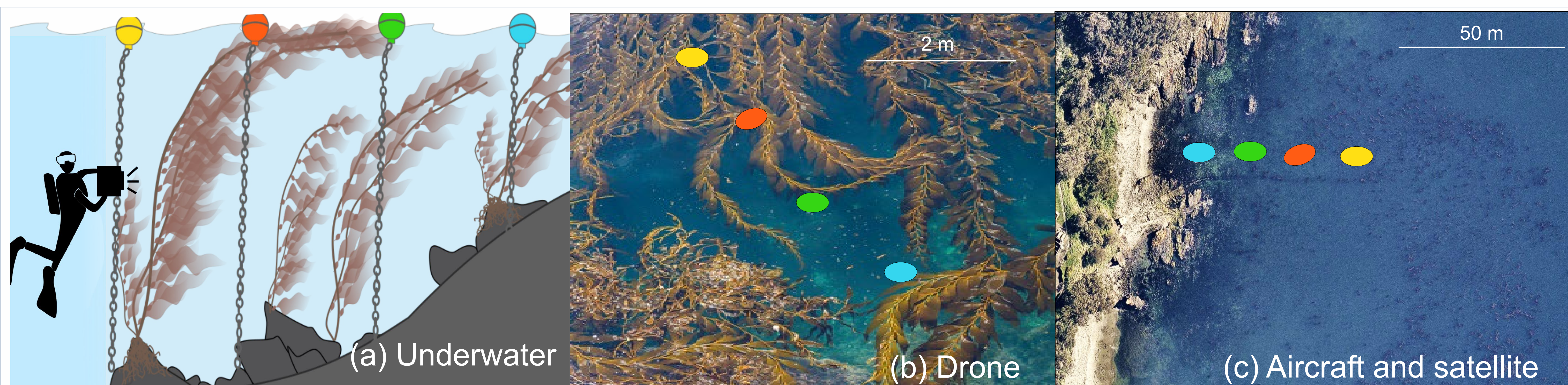
Figure 2: Proposed methods to: (a) collect and transfer field based kelp measurements of kelp extent and biomass; (b) along the transect line of surface buoys (marked by different colours); and (c) to high spatial resolution satellite data of kelp forests at two scales of observation. These data drive the models shown in Figure 3.
